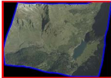
Figure 6 – footprint and bounding box of an orthoimage (respectively in blue and red)
